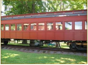
The 1902 wooden passenger car is in its final stages of restoration. The outside is complete except for the final paint. In side we have the newly installed seats of the era 1902, with a new hardwood floor.
